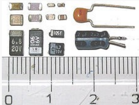
Modern capacitors, by a cm rule.
